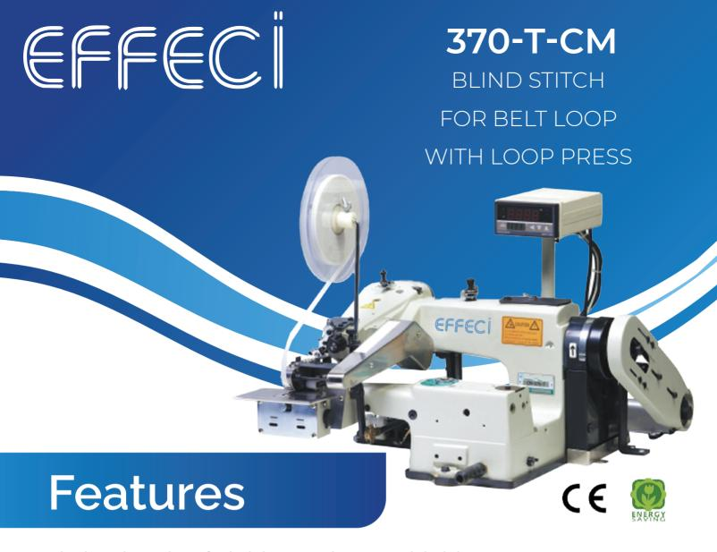
Blind stitch machine for belt loop production with belt loop press.
