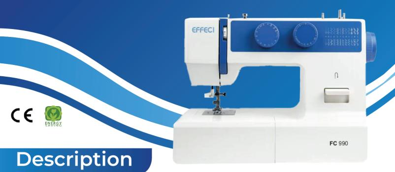
Mechanical free-arm sewing machine, 24 stitches, 4-step buttonhole, automatic needle threader, oscillating hook, stitch length (max 4mm) and zigzag width (max 5mm) adjustment, feed dog embroidery plate, LED light, twin needle spool pin, stitch tableau and speed up to 800rpm.
