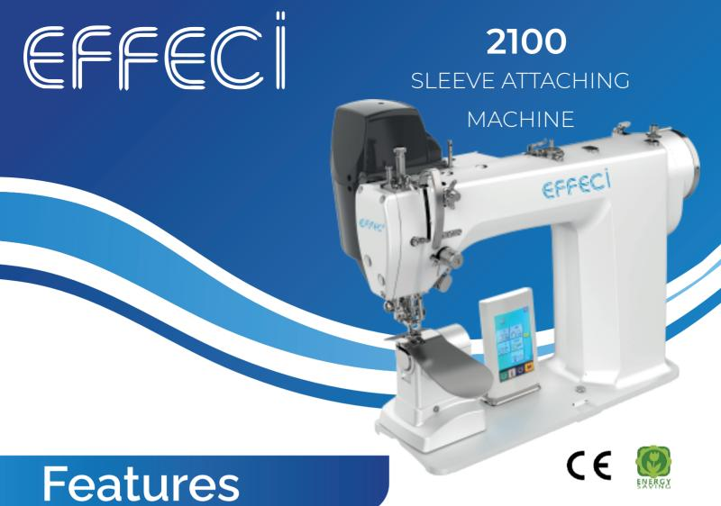
Sleeve attachment machine post bed type and direct drive motor. Feeding with 2 independent lower and 2 upper belts, central foot with alternating movement, thread trimmer, bartack and presser foot lifter. Dry head without lubrication. Equipped with a pedal to vary the speed scale with manual setting, touchscreen panel that allows you to program the different sections of the armhole.
